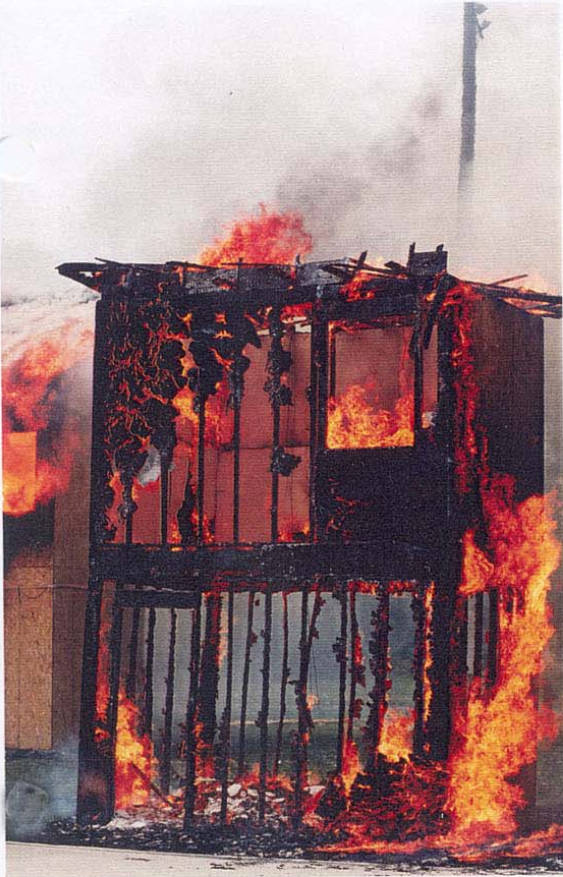
Structure with no insulation collapsed 40:10 after ignition.
