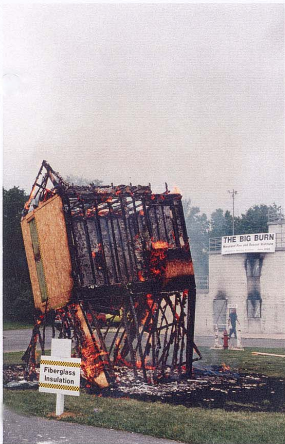
Structure with fiberglass insulation collapsed 42:26 after ignition.
